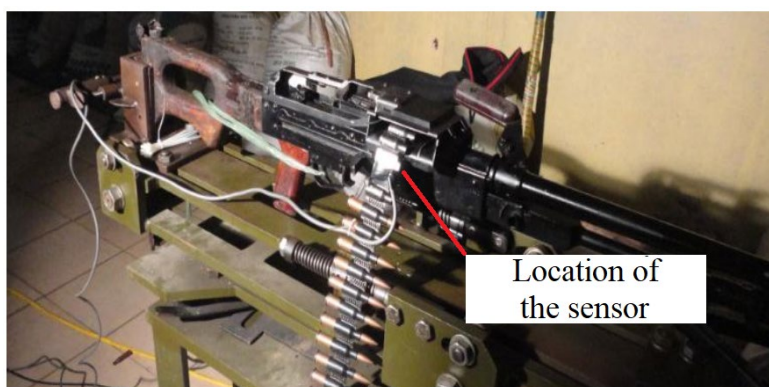
Figure 14 – Simulated belt link installed on a machine gun ammunition belt
