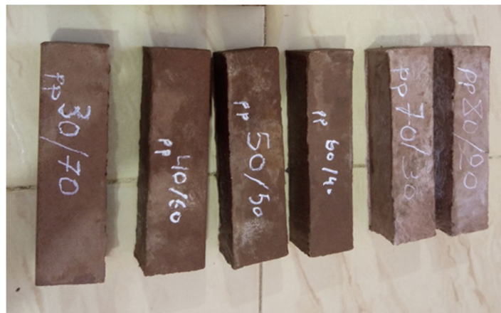
Figure 11 – Plastic brick specimens (prismatic).
