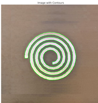
Figure 11 – Circular coil image after contour detection and drawing
