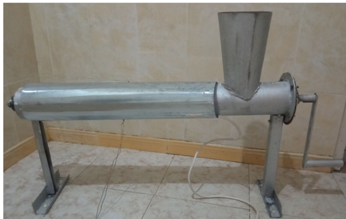
Figure 8 – Manuel plastic brick extruder
