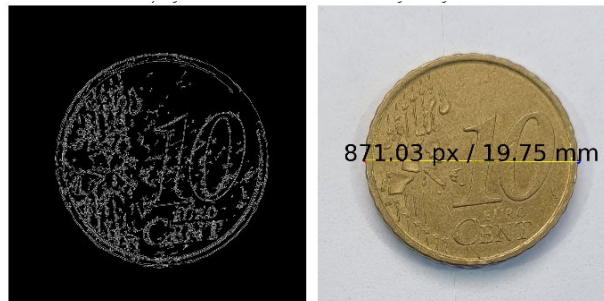
Figure 13 – Coin image processing for pixel-to-millimeter conversion
