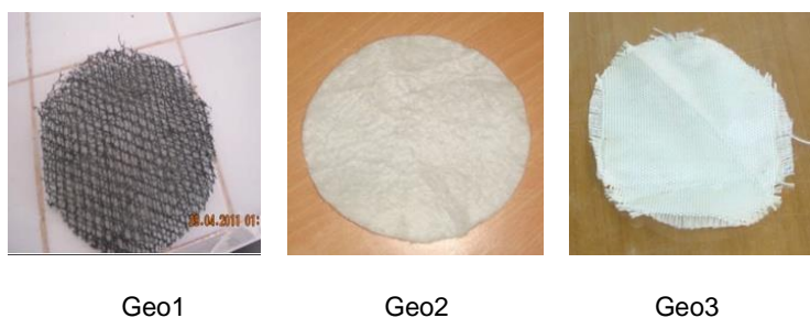
Photo 1 – Geosynthetics (Geo1 is a geogrid, Geo2 is a non-woven geotextile and Geo3 is a woven geotextile)
