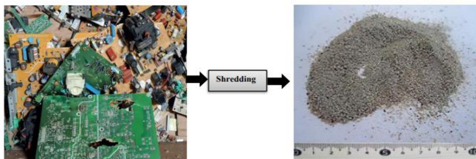
Figure 2 – Photographs of the electronic boards of a cathode ray tube before and after shredding
