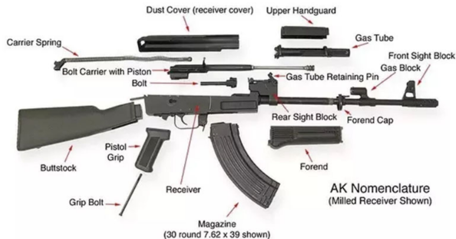
Figure 2 – Main components of the AK submachine gun
