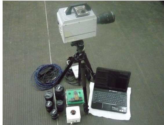
Figure 26 – SA1.1 High-speed camera system
