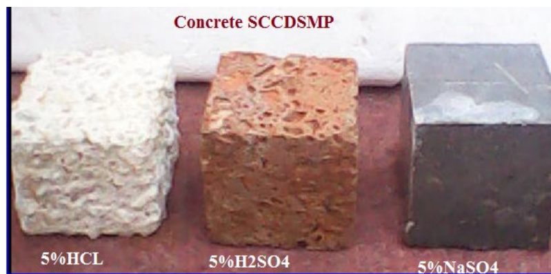
Figure 13 – Condition of the cubic specimens of SCCDSMP concrete after etching at 28 days
