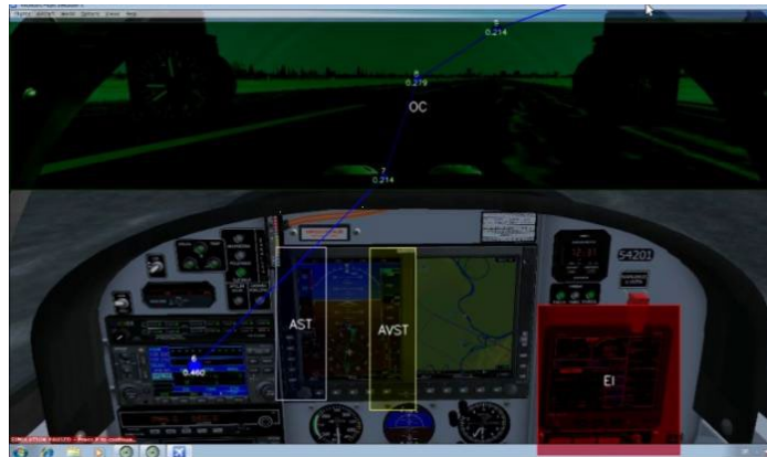
Figure 16 – Appearance of the cockpit of the Lasta aircraft in the Microsoft Flight Simulator and 4 AOIs for which the instrument scanning schedule was recorded in the paper Vlačić et al. (2020)
