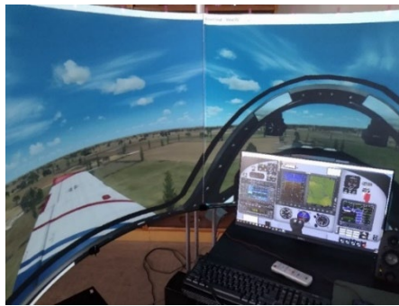
Figure 8 – Extension of the field of view to the PCATD trainer for the Lasta aircraft
