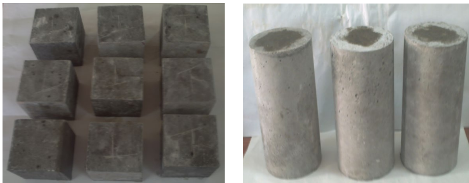
Figure 2 – 7.7.7 cm cubes for durability tests and 11.22 cm cylinders for compressive strength tests
