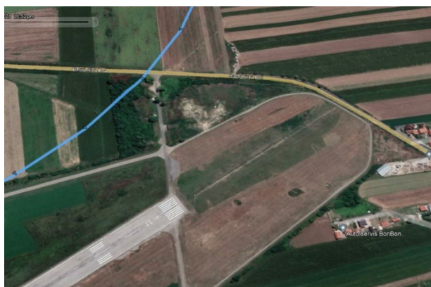
Figure 13 – Recorded trajectory from a simulated flight in the SKY Demon app and the FSX add-on for the Lasta aircraft. The trajectory is recorded in the Google Map extension .gpx
