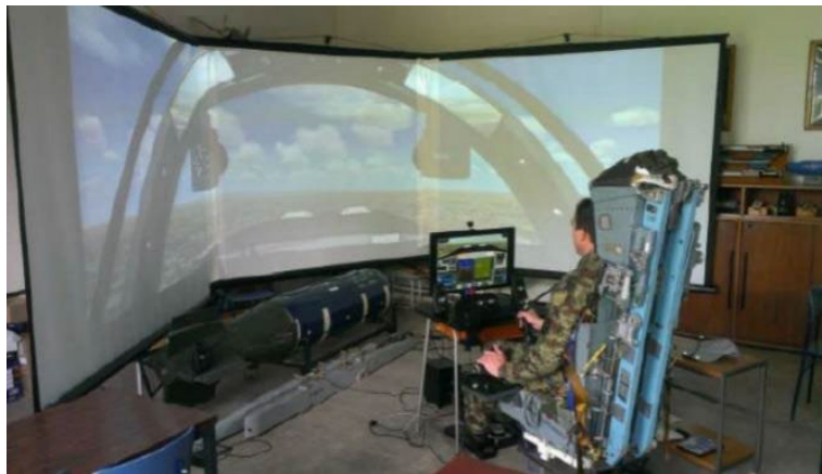
Figure 3 – PCATD trainer for the Lasta aircraft with a 90° field of view
