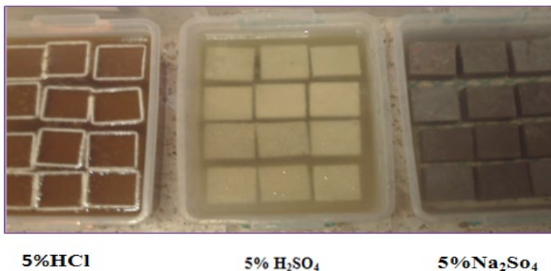
Figure 7 – Cubic test tubes immersed in acid solutions
