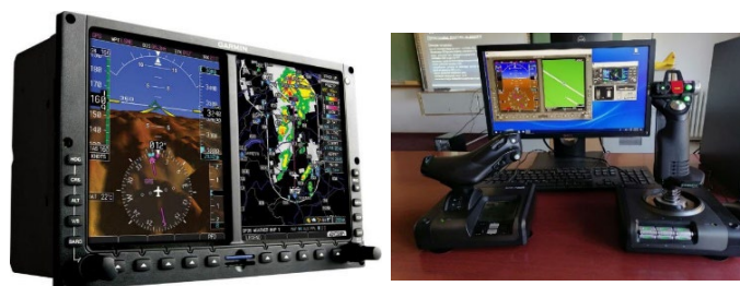
Figure 1 – Garmin 500, the instrument found in the Lasta aircraft (left), and a desktop trainer with Garmin software used to train cadet pilots
