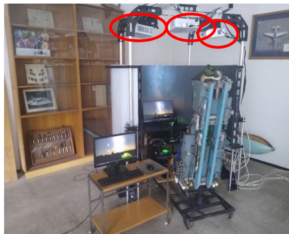
Figure 7 – Modernized PCATD trainer for the Lasta aircraft and the position of the short-throw projectors (rounded positions)
