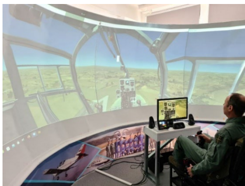
Figure 10 – PCATD trainer for the Gazelle helicopter with analog instruments and with a projection surface in the form of a spherical section measuring 150^{\circ} \times 60^{\circ}
