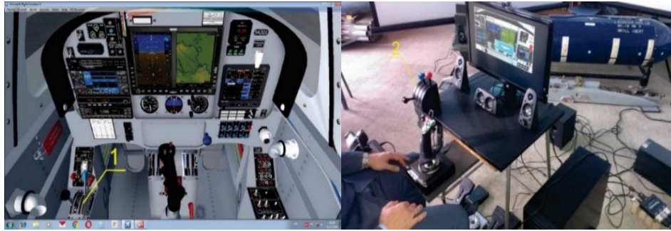
Figure 5 – Controls in the cockpit of a Lasta aircraft (left) and in the physical setup of the PCATD trainer (right)
