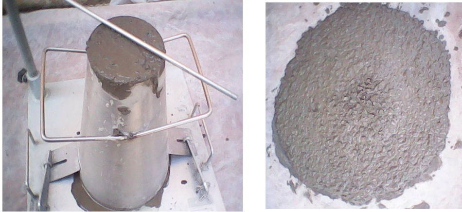
Figure 3 – Abrams cone slump/spread test
