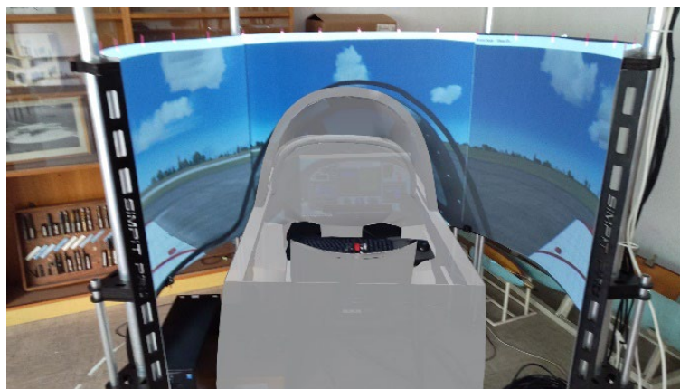
Figure 4 – PCATD trainer for the Lasta aircraft with a field of view of 270°
